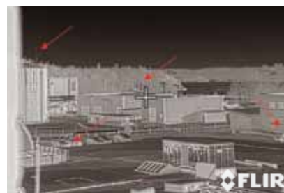
DDE applied - all targets can be observed simultaneously
